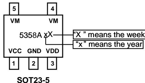
Figure 1. PIN Configuration
