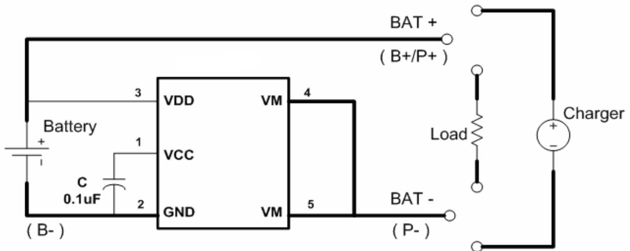
Fig 6 PL5358 in a Typical Battery Protection Circuit
